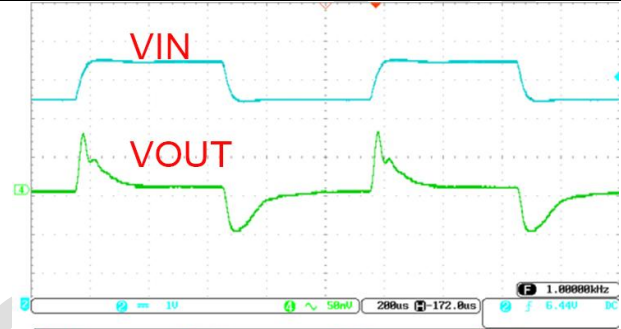
Figure 2 Line Transient (VIN=from 5.6V to 7V to 5.6V IOUT=150mA)
