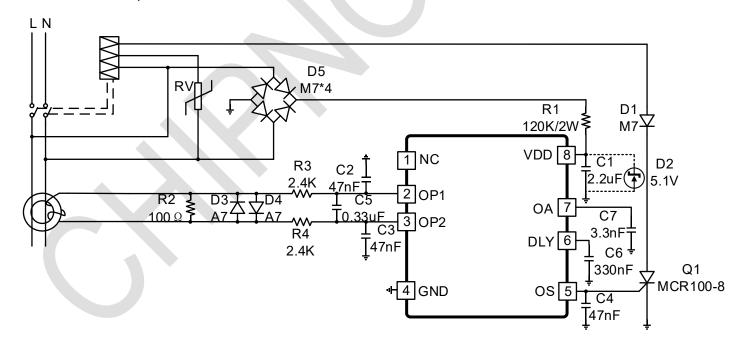
In the above application circuit diagram, T0 is the ZCT used to induce the leakage current on the power supply line, R2 is the leakage protection action sensitivity adjustment resistance, the value of the resistance is related to the leakage current required to act and the turn ratio of the ZCT,the action sensitivity inside the CN54123A/B/C/D is 4.95mV, then ideally
