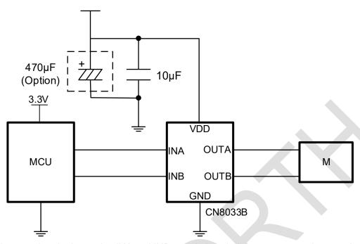
Please make sure that the input pins INA and INB remain low during power-up and power-down.
